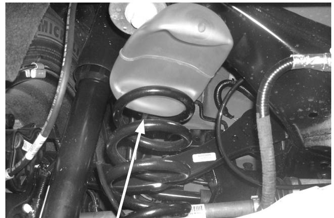
Insert cylinder with stem pointing down
