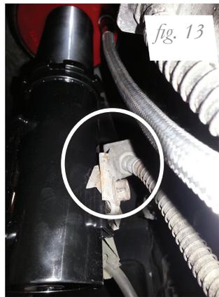
5. Fully compress the suspension using a jack. With the suspension compressed, review the best routing for the leader hose that is clear of all suspension components and axle. Routing should also allow for the suspension to extend without kinking or pulling the line tight or rubbing on other components. Following the brake line routing is often a good place to start. Check clearances to all other components.
