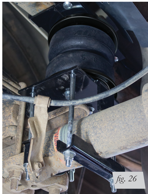
Right side (passenger): front view of installation.
