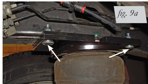
Left hand assembly (driver side) attached with carriage bolts (R), flat washers (M) and nylon lock nuts (U). Torque to 31 lb.-ft.
