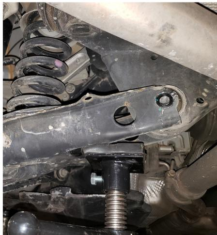
4. Remove the coil spring and rubber spring seats.
