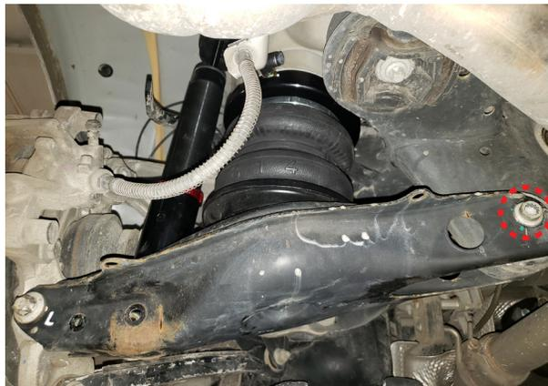
5. Attach the shock and end link to the control arm. Do not torque until at desired ride height with load.
