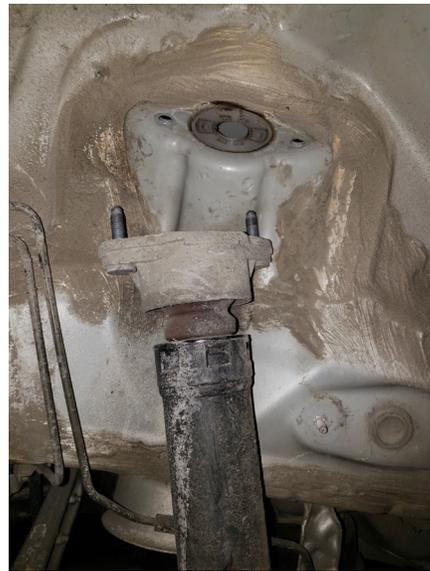
6. Disassemble the upper mount from the shock rod.
