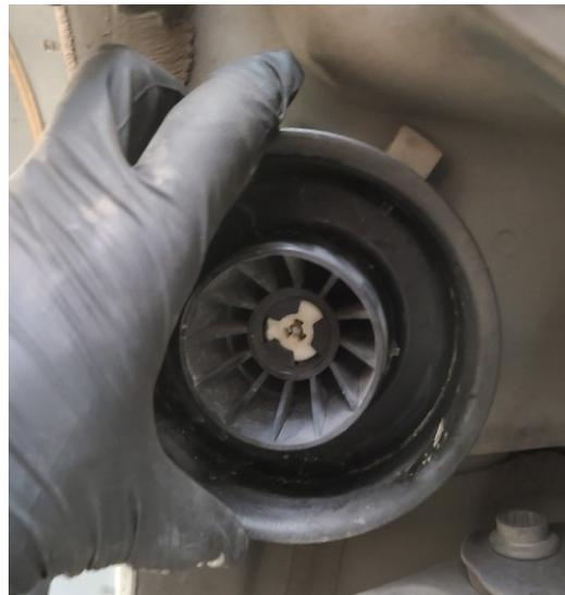
5. Unfasten the shock upper mount from within the luggage compartment. Remove the shock assembly.
