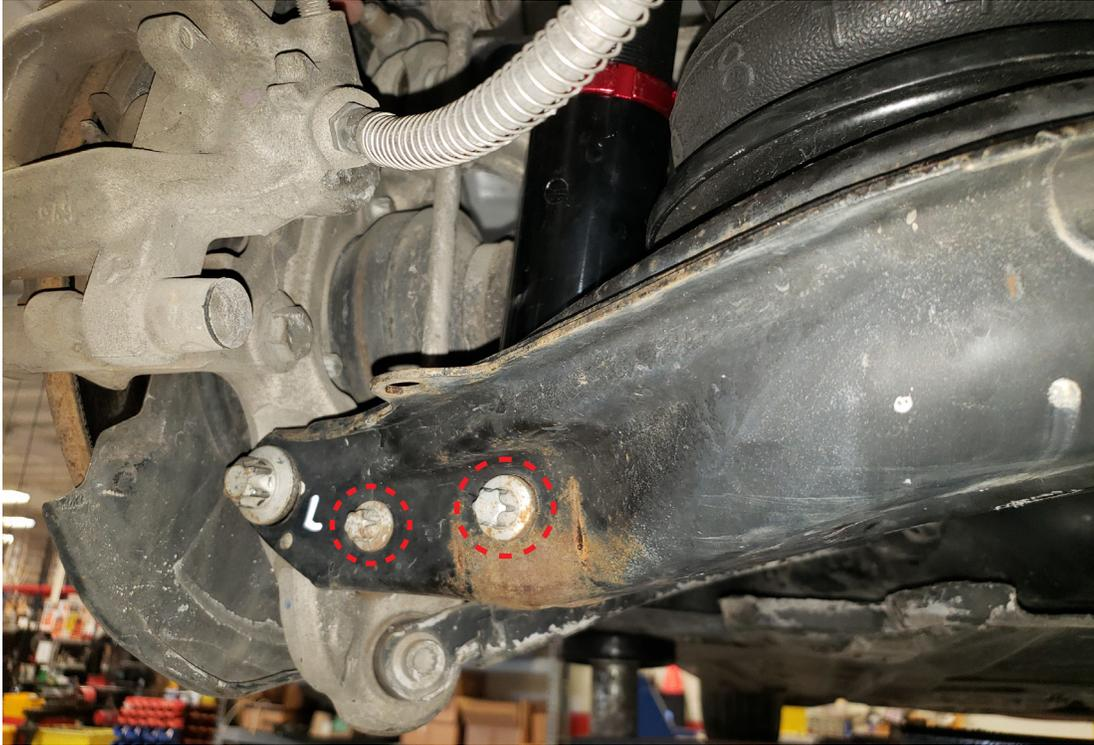
6. Secure the air spring assembly to the lower control arm with the centering spacer, lock washer, and bolt. Torque the bolt to 27Nm (20 lb.-ft.)
