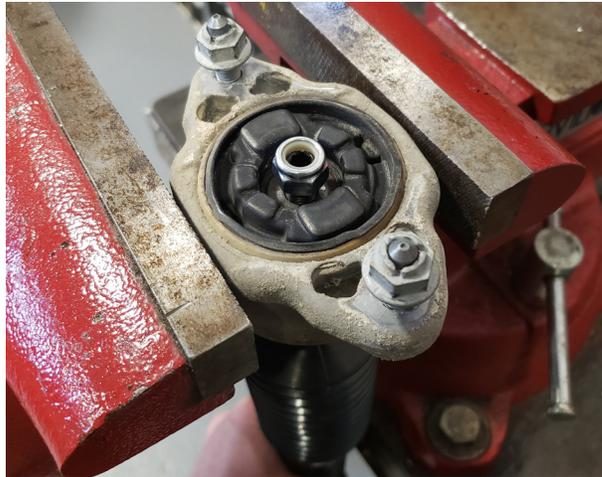
3. Install the shock assembly to the chassis and torque upper mount nuts to 15Nm (11 lb.-ft.), release pressure and continue torque to 35Nm (26 lb.-ft.).
