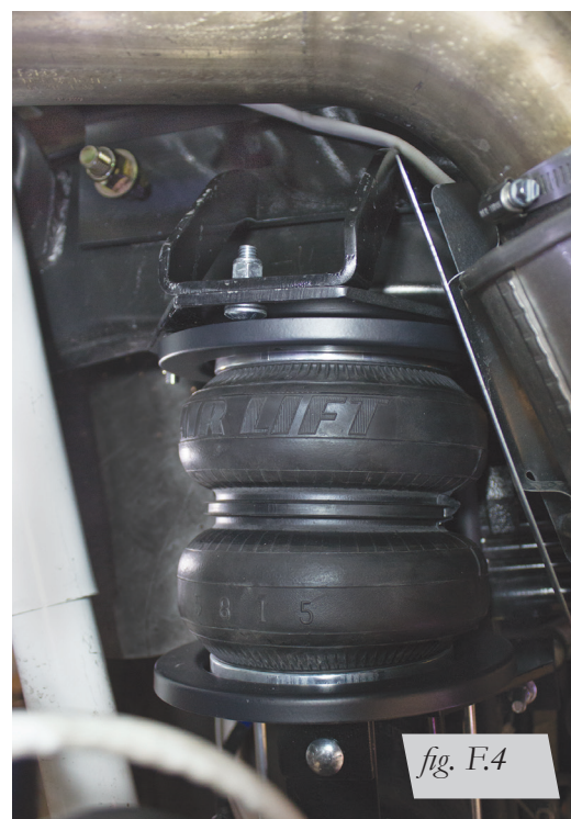
Right-hand installation from the middle.
