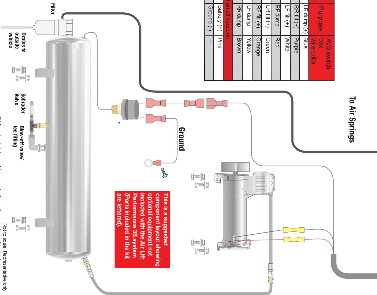
This is a suggested component layout showing optional equipment not included with the Air Lift Performance 3S system (Parts included in the kit are lettered).
